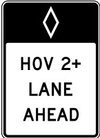
Figure 2.6: Reserved lane sign In this example, the lane is reserved for high-occupancy vehicles (HOV) carrying two or more people.
