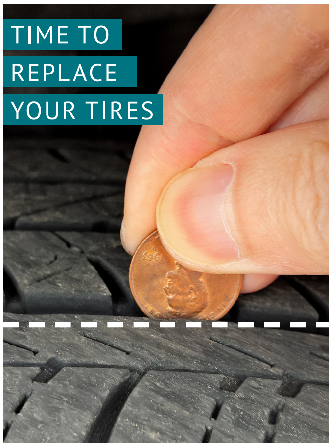
Figure 3.1: Check your tire tread with a penny
